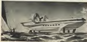
A hydrofoil still on the drawing board: in addition to a gas turbine it has air screws, too.
